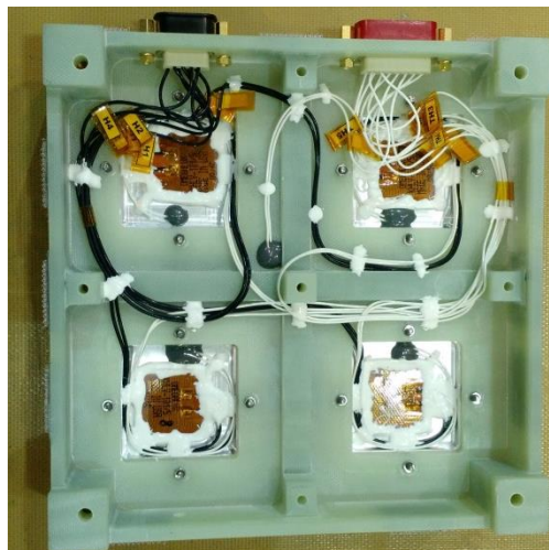
Figure 6. Heaters and thermistors placed inside the experiment assembly.
